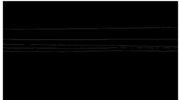
After skeletonization, we have a binary mask with all the horizons annotated as 1px wide lines.
